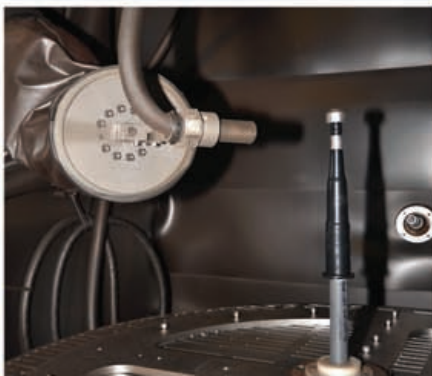
Robotic ID/OD Shot Peening
